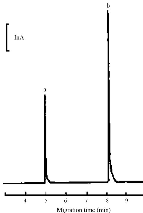
Fig. 3. Electropherograms of a standard solution containing  $5 \times 10^{-5}$  M aminoheterocycle and azabicyclic under the optimal CZE-AD conditions: a, azabicyclic; b, aminoheterocycle.
