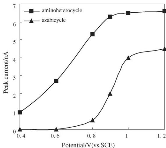
Fig. 2. Hydrodynamic voltammograms for aminoheterocycle ( $5 \times 10^{-5}$  M) and azabicyclic ( $5 \times 10^{-5}$  M); the CZE conditions are as the optimal.
